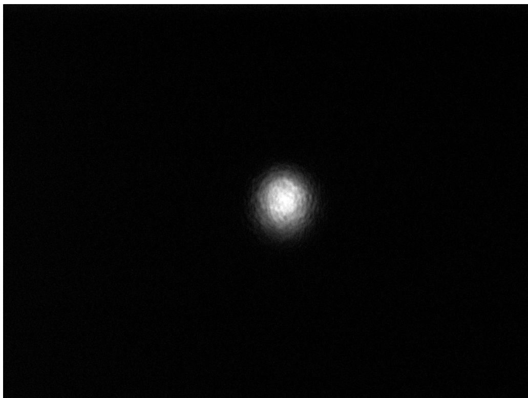
Figure 1: IR image of laser beam profile. Images were compiled to determine the vertical position of the beam versus time when using the rotation macro.
