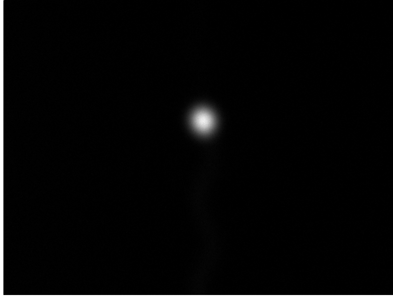
Figure 2.7: An image of the electron beam captured by the CCD imaging system. Brighter, higher intensity pixels show the location of the beam.
