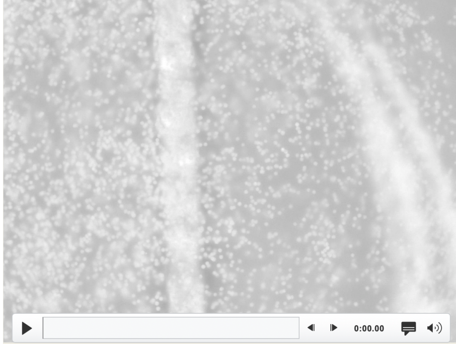
Figure 2.11: The movement of polyethylene microspheres in a high level of castor oil when 5\text{ kV} is applied to the conducting copper trace. The liquid level recedes from the trace as it is pushed away, acting as a weak field seeker.
