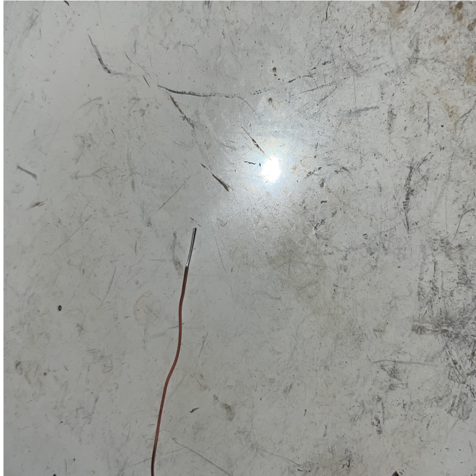
Figure A.1: Exposed teflon layer after the removal of the copper layer.
