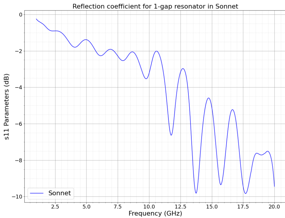
Figure 3.9: Reflection coefficient vs. frequency for the one-gap resonator of figure 3.7a.
