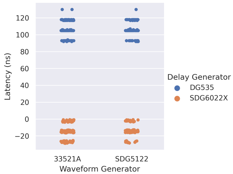
Figure 3.12: Plot of intrachannel latencies for combinations of waveform and delay generators.
