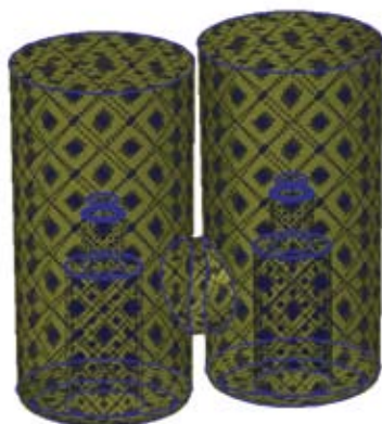
Cavity resonator showing the default Perfect Electric Boundary on all outer solution space surfaces
