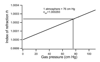
In the lab you will measure the change in interferometer fringes  $\Delta m$  as the air pressure p is varied.
