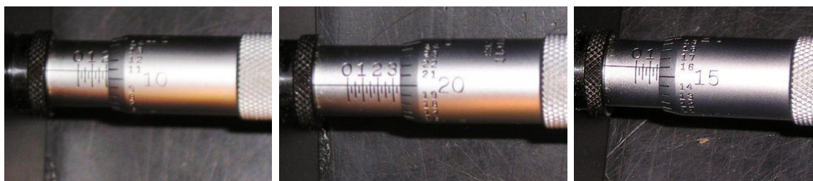
Figure 3: Micrometer readings. The coarse division equals to 100 \mu\text{m} , and smallest division on the rotary dial is 1 \mu\text{m} (same as 1 micron). The final measurements is the sum of two. So, from left to right, the figures above show 211 \mu\text{m} , 345 \mu\text{m} , and 166 \mu\text{m} .
