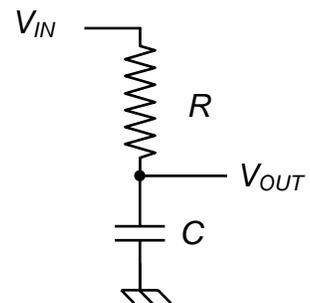
2c. (Same set-up) Set the function generator to sinusoidal output at  $\omega=1/RC$  and measure the magnitude of  $V_{in}$  and  $V_{out}$ . Do you get what you expect?
