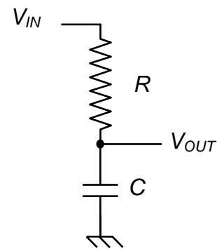
$$\left| \frac{V_{out}}{V_{in}} \right| = \left| \frac{1/i\omega C}{R + 1/i\omega C} \right| = \left| \frac{1}{1 + i\omega RC} \right| = \frac{1}{\sqrt{1 + (\omega RC)^2}} = \sin(\phi) \quad (2)$$
