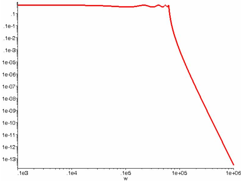
This Chebyshev filter uses  $C_1 = C_5 = 1.125 \mu\text{F}$ ,  $C_2 = C_4 = 1.486 \mu\text{F}$ ,  $C_3 = 1.505 \mu\text{F}$ ,
