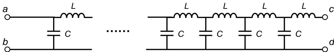
If the LC ladder is infinite and has an impedance  $Z_0$ , then if we add an extra LC ladder “rung”, the total impedance should not change, and we obtain the following relation
