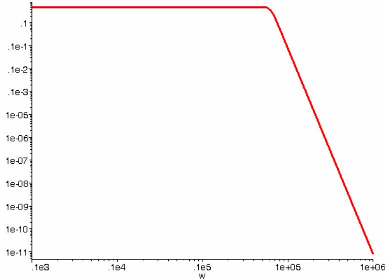
This Butterworth filter uses  $C_1 = C_5 = 0.6946 \mu\text{F}$ ,  $C_2 = C_4 = 3.0642 \mu\text{F}$ ,  $C_3 = 4 \mu\text{F}$ ,  $L_1 = L_4 = 5 \text{ mH}$ , and  $L_2 = L_3 = 9.397 \text{ mH}$ . Butterworth filters have a very flat pass-band, and a reasonably regular phase change across the knee of the curve.
