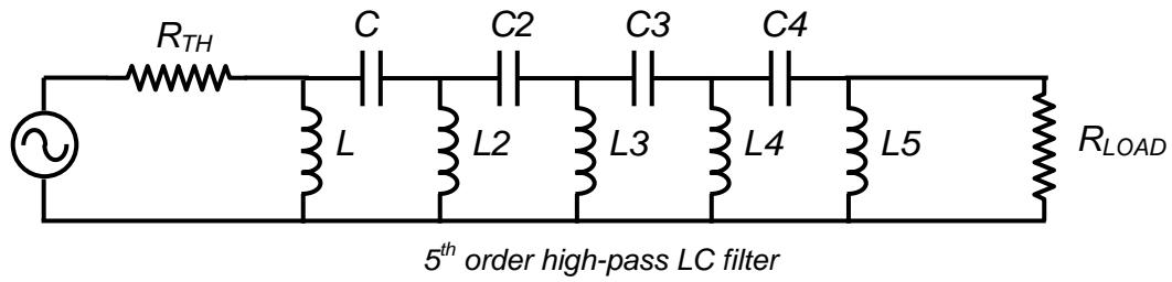
The algebra required for computing the gain and phase Bode plots for these filters is generally quite cumbersome, and a computer program (i.e. Maple or Excel) is generally useful for helping with the design. A number of web-applets can also be found on the internet for determining all the inductor and capacitor values that will produce the required filter performance.
