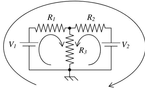
The sign conventions are that the voltage increases across a power supply and decreases across a resistor in the direction of current flow. The direction of current flow should be the same as the one defined for the Point Law. In our example circuit there are three loops that could be considered. From these three loops we could write down three relationships:
