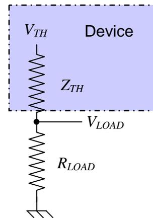
A special case is when there isn't any load applied (i.e. option 1 above, where  $R_{LOAD} = \infty$ ) then the output is simply  $V_{TH}$ . From the results of these two measurements we can solve for  $R_{TH}$ .
