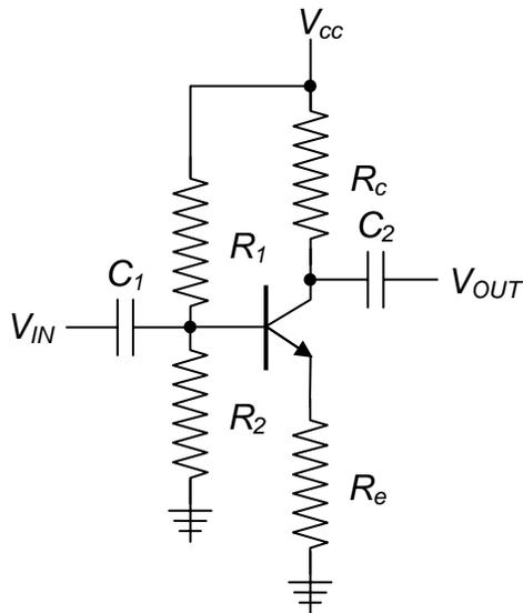
$$I_{Bias} = V_1 / R_1 = V_2 / R_2 .$$
