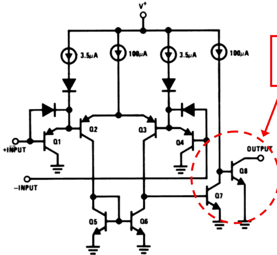
Output is configured for use with a pull-up resistor
