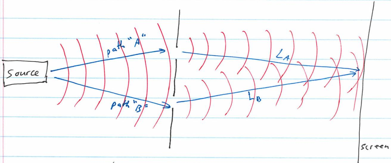
$$\text{phase accumulated along path } A = \phi_A = 2\pi \frac{L_A}{\lambda} = 2\pi [L_A \text{ mod } 1]$$
