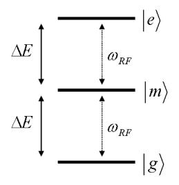
An RF magnetic field with frequency  $\omega_{RF}$  is applied to the atom resulting in a (resonant) 2-level Rabi frequency of  $\Omega$  for both the  $|g\rangle \leftrightarrow |m\rangle$  and  $|m\rangle \leftrightarrow |e\rangle$ . The  $|g\rangle \leftrightarrow |e\rangle$  transitions are forbidden.
