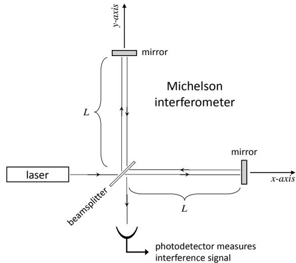
*Michelson interferometer for detecting gravitational waves. The two mirrors and the beamsplitter are suspended so that they act as free masses.*
