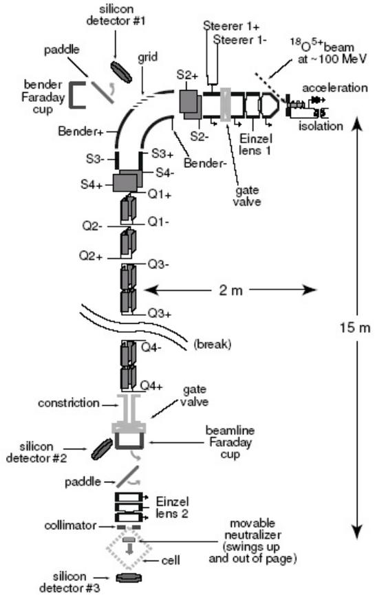
Figure 2: New beamline for transporting Francium away from the target area.
