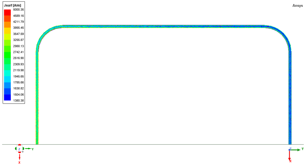
Figure 4.2: Current density distribution from a 6.8 GHz input at left port signal plotted on a single microwave trace.
