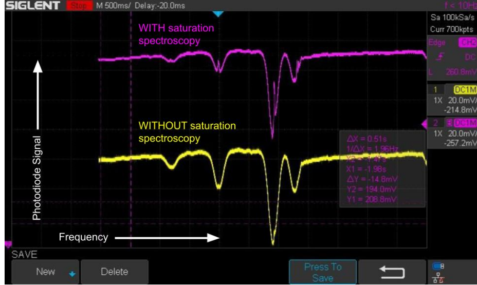
Figure 3.5: Oscilloscope frequency vs. potential data of Doppler broadened absorption lines of rubidium with and without 5P saturation spectroscopy dips. Above (pink) graph displays data with laser saturated absorption spectroscopy features, below (yellow) graph displays data without.
