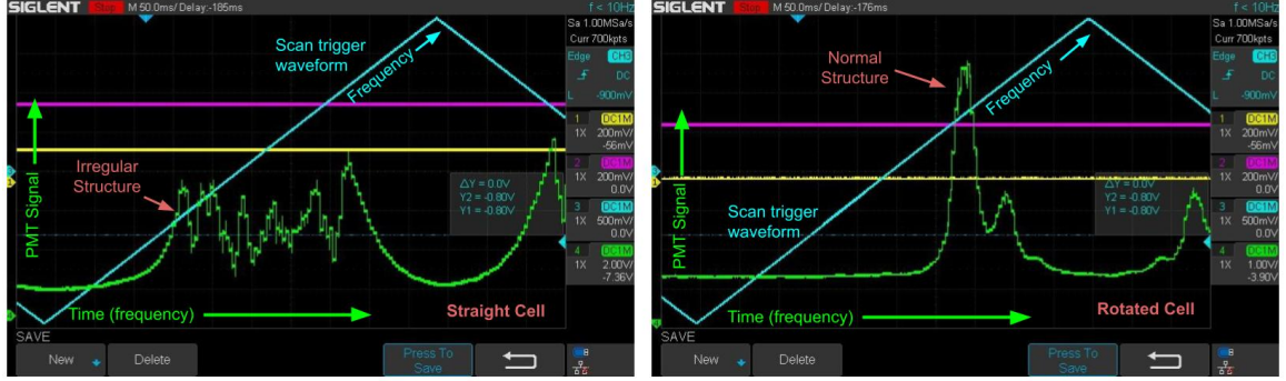
Figure 4.4: Oscilloscope PMT signal vs. time (frequency) data of 5D_{5/2} fluorescence spectroscopy of rubidium-85 in a vapor cell. Left side displays data when vapor cell is not rotated, observing extremely irregular photopeak structure. Right side displays data when vapor cell is rotated, observing only three photopeaks.
