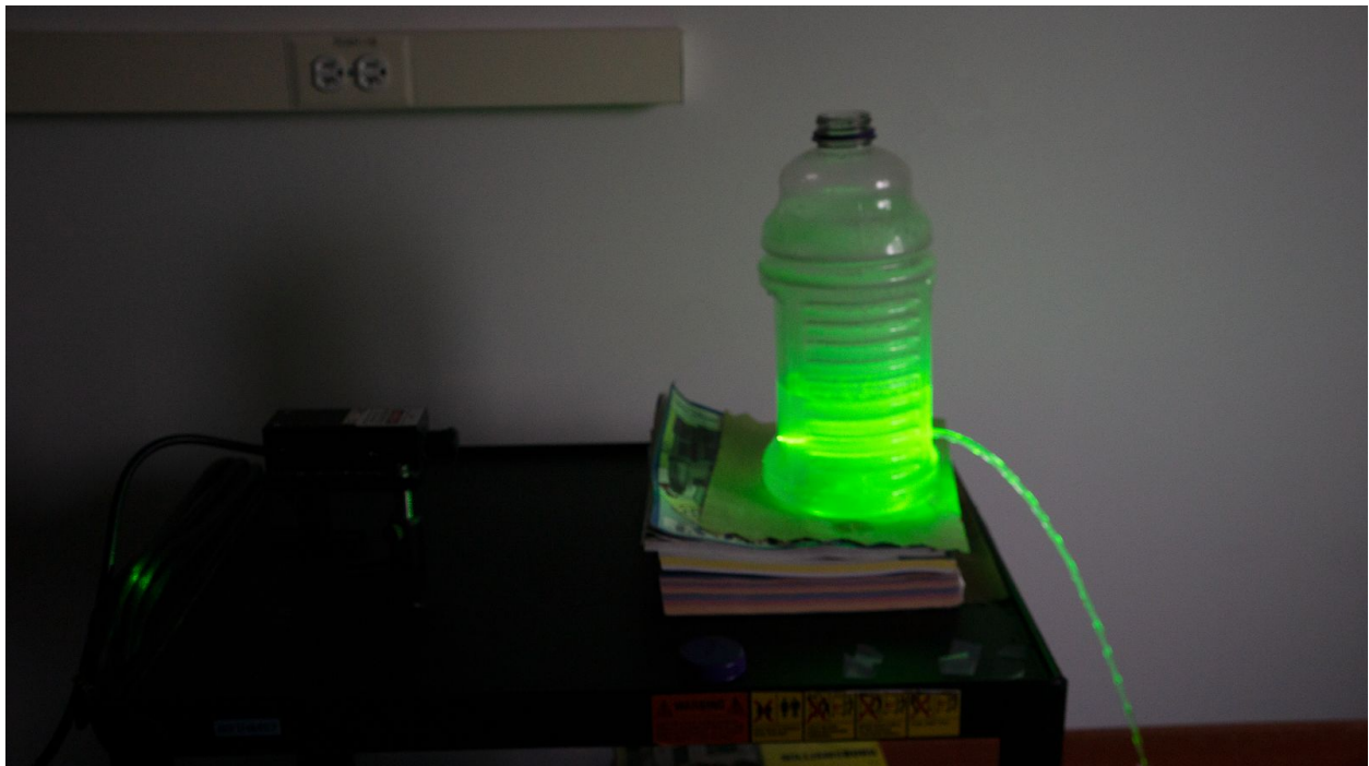
Figure 12: Setup of Laser through the Bottle with Hole
