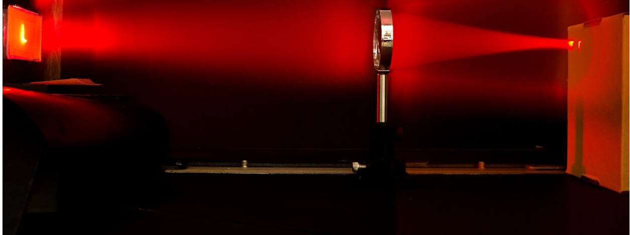
Figure 5: The Laser Method. The laser beam goes through the diffuser, letter L, and lens to appear on the screen. The beam has been made visible with the use of a hand held cardboard screen and a long exposure.
