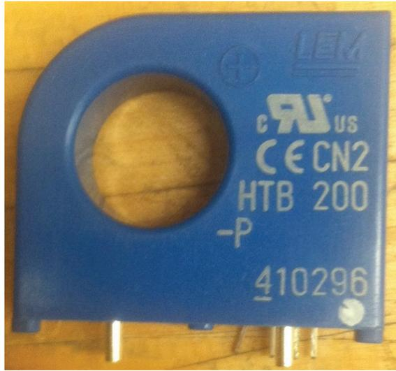
Figure 11: Current Sensor: The sensor will be implemented to provide an ‘enable’ signal to the D-Latch gate, thereby impeding any switching while current is flowing in the coil.
