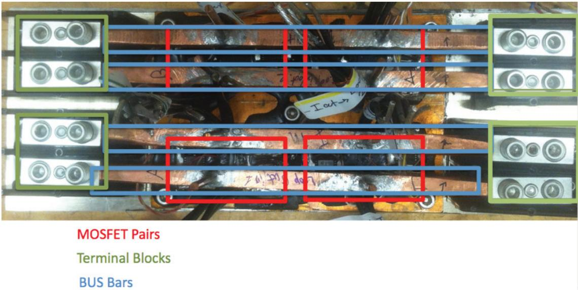
Figure 8: The switch core as seen from above. This is the physical implementation of the layout sketched in Fig. 6.
