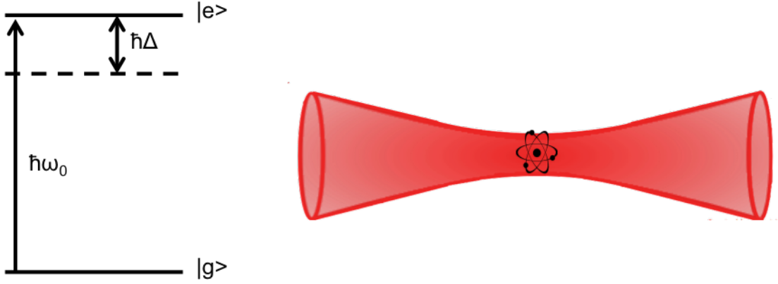
FIG. 3.1: Two-level energy diagram. (left) A two-level atom is assumed to have two energy levels: a ground state |g\rangle and excited state |e\rangle separated by energy \hbar\omega_0 . For optical dipole trapping, a far off-resonance detuned wavelength is chosen, represented by energy detuning \hbar\Delta . (right) A red-detuned beam results in atoms being confined in the high intensity region of the beam, often formed simply by focusing the beam. Note that \hbar\Delta in the left figure is shown with \hbar\Delta < 0 (red-detuning) to match the right figure.
