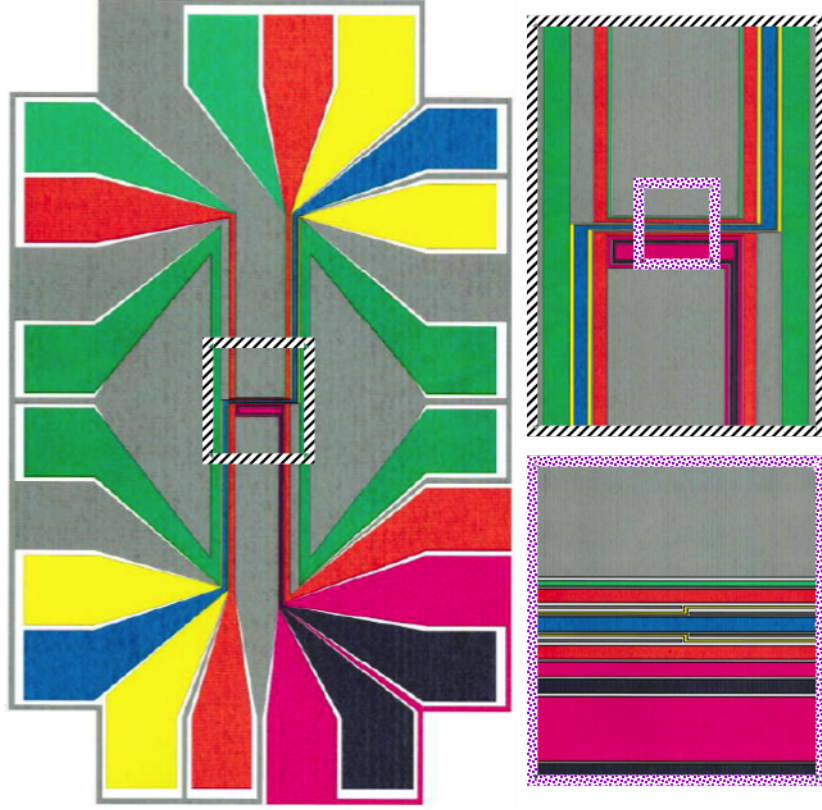
FIG. 2.7: Atom chip metalization. The left image illustrates the various wire patterns on our atom chip generously donated by the Thywissen Lab at the University of Toronto. A zoomed in image of the center portion, outlined in black/white, is shown in the upper right corner. Here the z-wire, shown in blue, is very evident. Further zooming in shows further structure in the bottom right image. For the work carried out in this thesis, the blue Z-wire trace is used for trapping and one of the red U-wires is used for RF evaporation.
