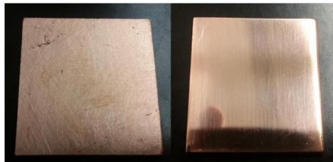
Figure 4.6: Copper Plate Before and After Polishing
