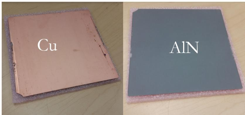
Figure 4.1: Both Sides of CERcuits Substrate Candidate
