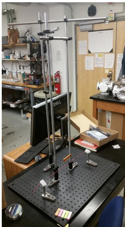
Figure 3.2: Pendulum with Horizontal Wire Geometry
