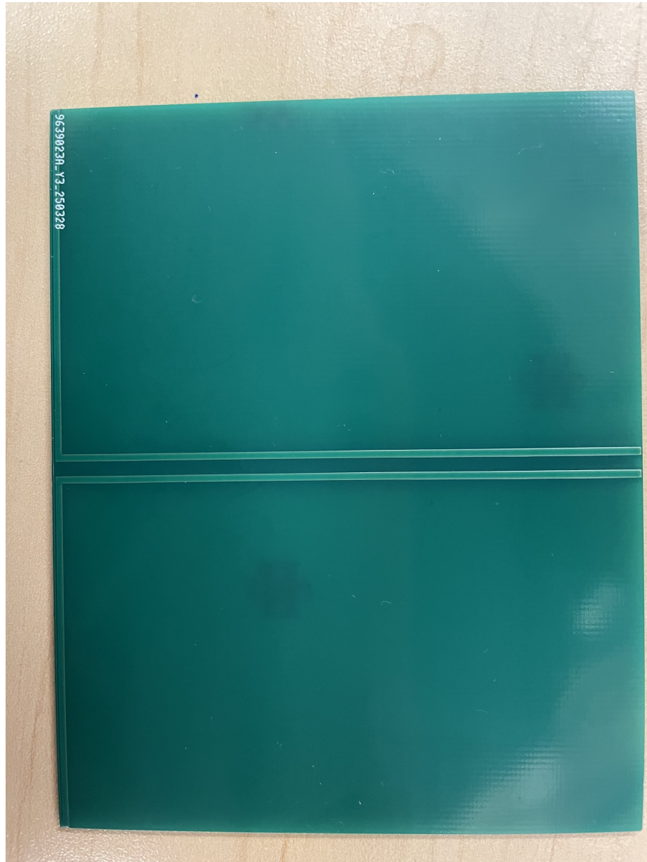
Figure 4.6: The PCB from JLC PCB before it was carved or wires soldered to it. The light green lines are the copper with a thin plastic coating overtop it.
