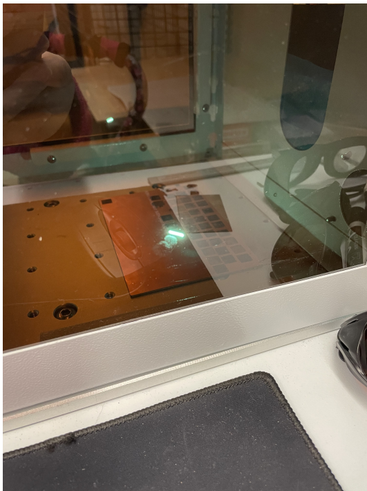
Figure 4.4: The Triumph laser cutting (and burning) into the PCB.
