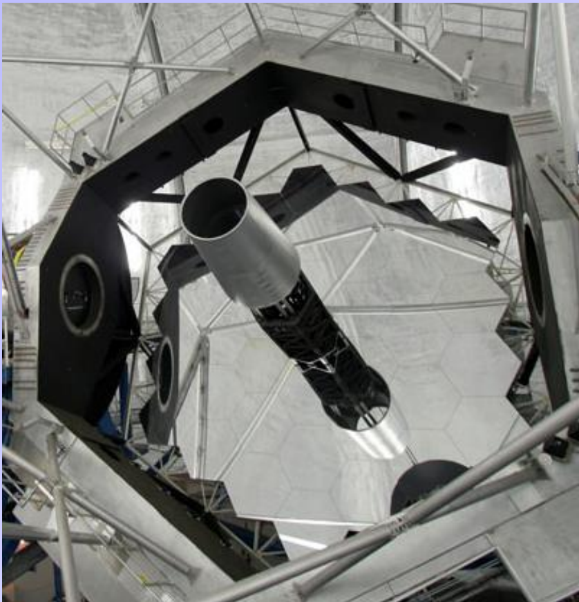
36-segment mirror of the Keck telescope (Hawaii)
