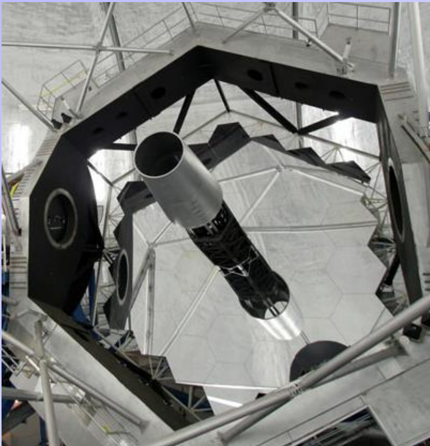
36-segment mirror of the Keck telescope (Hawaii)
