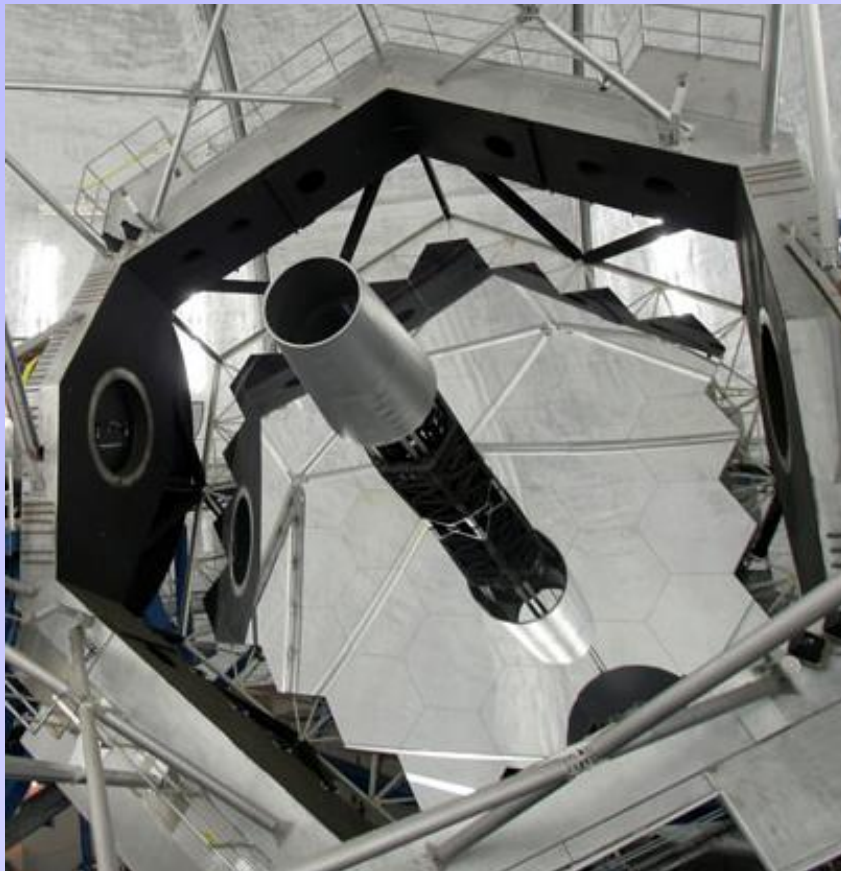
36-segment mirror of the Keck telescope (Hawaii)
