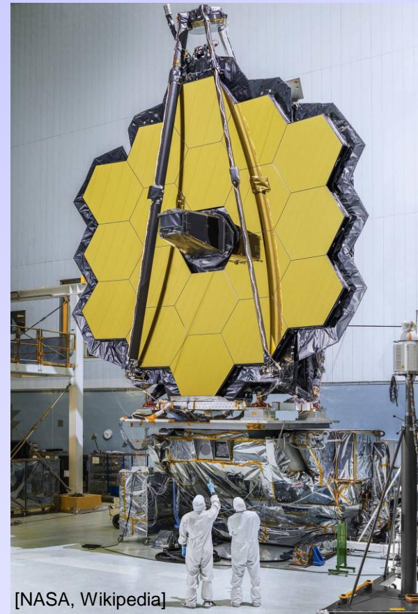
18-segment mirror of the James Webb Space Telescope.
