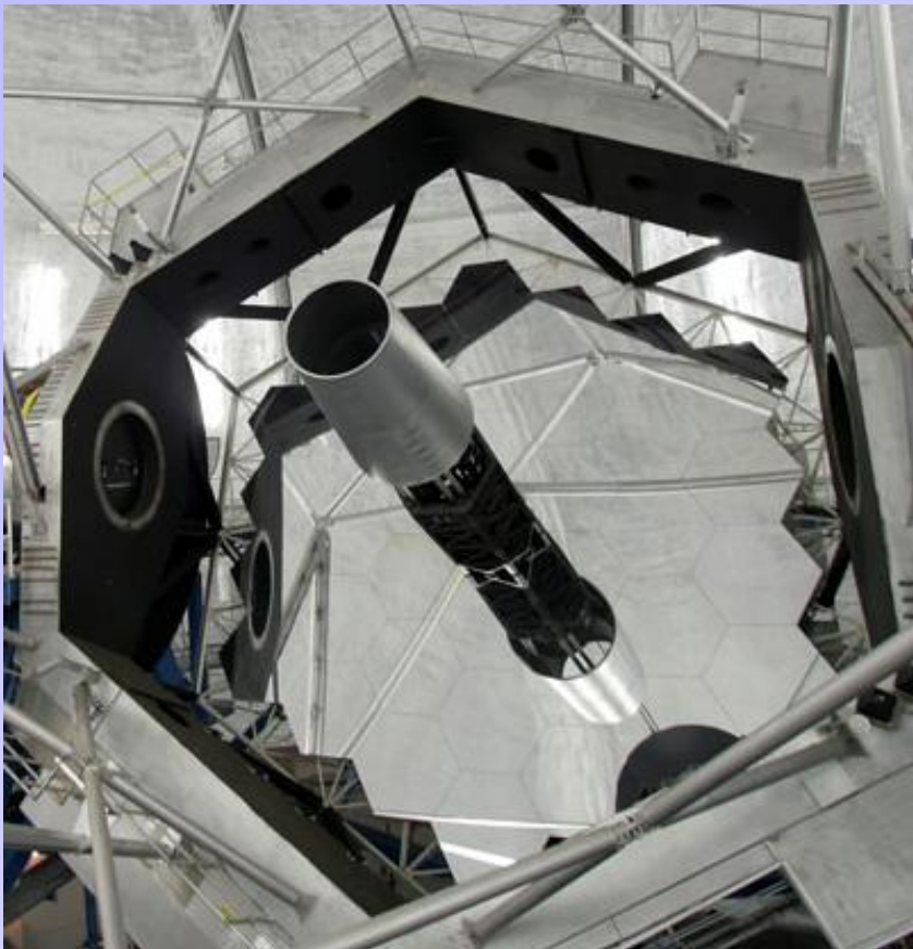
36-segment mirror of the Keck telescope (Hawaii)
