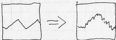
Iraha figured out that we needed to turn the photodetector, and when we did this we saw the plain triangle wave again. From there, I began to turn the temperature up, and maxed the peltier out at  $36.4^{\circ}\text{C}$ . At this temperature, we saw the resonances with approximately  $1.70\text{ mA}$ .
