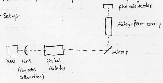
• We had to add an additional convex lens to help collimate the laser, because the focus was very short.
