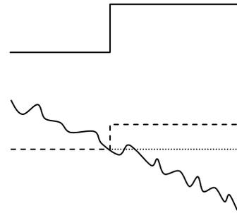
Figure 2: When the output makes a transition (top), the reference level can be shifted (dashed) using positive feedback to prevent extra transitions as the input on  $V_-$  (bottom) makes multiple transitions across the original reference voltage on  $V_+$  (dotted line).
