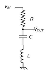
**Design Exercise 3-4:** Calculate  $V_{out}$  as a function of  $V_{in}$  in the RLC circuit depicted on the right, using the formulas for  $Z_R$ ,  $Z_C$ , and  $Z_L$  (do not use Maple / Mathematica / MATLAB / MathCad for these calculations and show all steps).  $V_{in}$  is a perfect AC voltage signal with a frequency of  $\omega$ .
