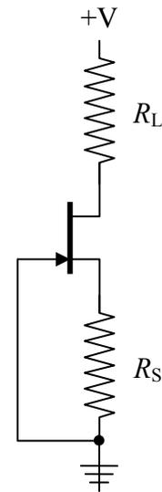
You can make this circuit an adjustable or *programmable constant current source* by adding a resistor between the gate and source to provide an offset (Figure 5). Since there is a voltage drop across the resistor the current is given by
