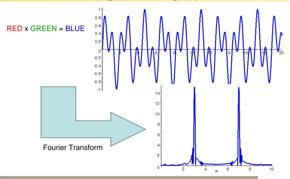
Digital mixing is does not produce any extra harmonics, unlike analog mixers
