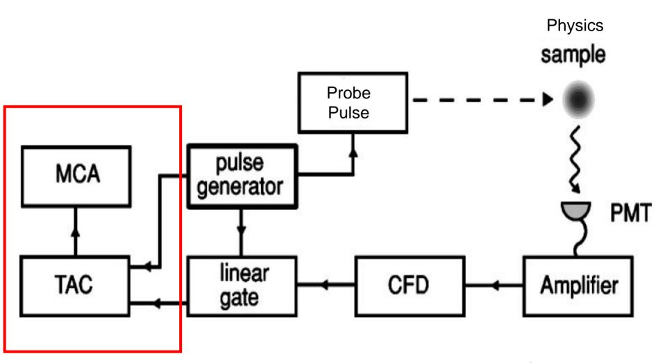
Histogram electronics ... easily replaced by an FPGA.
