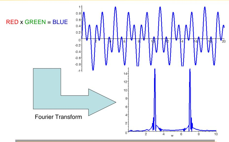
Digital mixing does not produce any extra harmonics, unlike analog mixers
