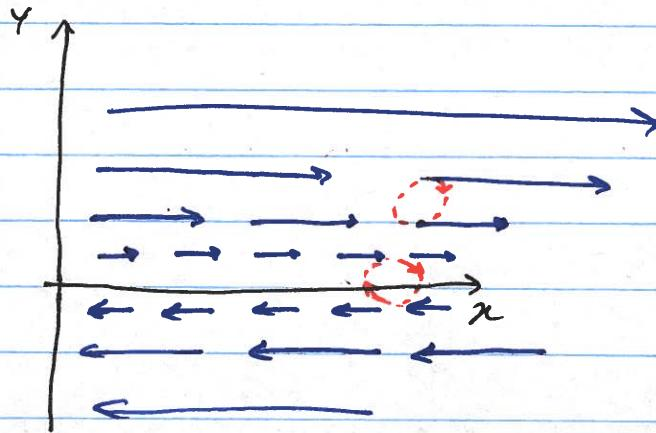
$$\begin{aligned} \vec{\nabla} \times \vec{C} &= (0, 0 - 0, 0 - c) \\ &= -c \hat{y} \neq 0 \end{aligned}$$
