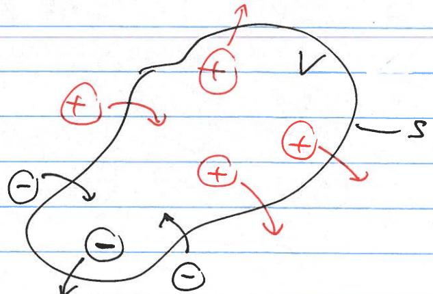
$I_{\text{out}}$  is also the total change in charge inside  $V$  per unit time.
