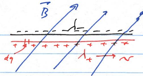
$$\vec{F}_{\text{magnetic}} = \int_{\text{wire length}} (\vec{v} \times \vec{B}) dq = \int_{\text{wire length}} (\vec{v} \times \vec{B}) I dl$$
