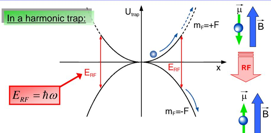
RF frequency determines energy at which spin flip occurs.
