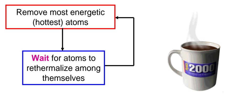
Wait time is given by the elastic collision rate  $k_{elastic} = n \sigma v$ Macro-trap: low initial density, evaporation time ~ 10-30 s. Micro-trap: high initial density, evaporation time ~ 1-2 s.
