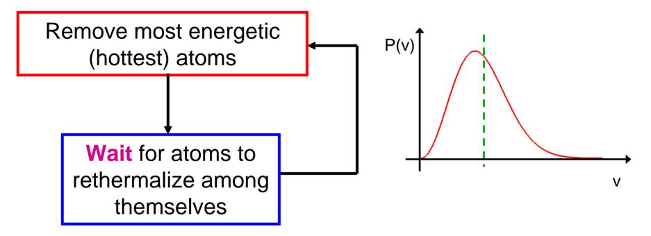
Wait time is given by the elastic collision rate  $k_{elastic} = n \sigma v$ Macro-trap: low initial density, evaporation time ~ 10-30 s. Micro-trap: high initial density, evaporation time ~ 1-2 s.
