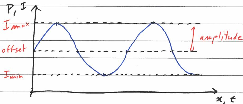
Def: Fringe visibility =  $\frac{I_{\max} - I_{\min}}{I_{\max} + I_{\min}} = \frac{\text{Amplitude of fringe}}{\text{Offset of fringe}}$
