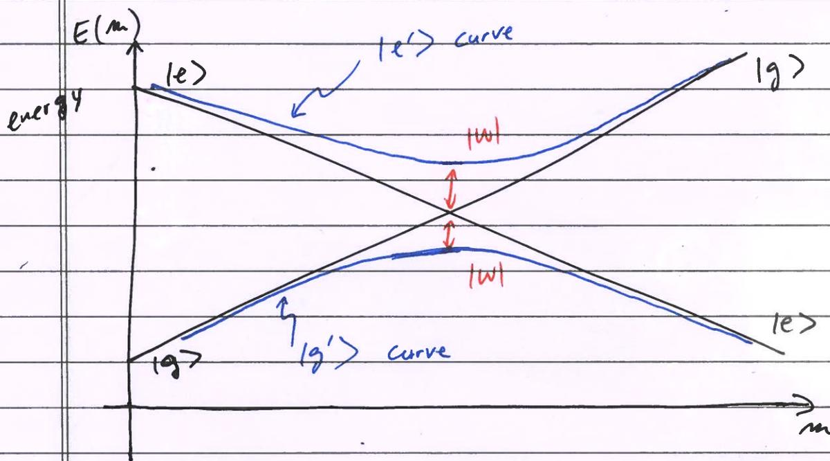
$\Rightarrow$  If 2 levels cross as a function of some parameter (i.e.  $m$  ... e.g. magnetic field, electric field, detuning, etc...), then, if there is any interaction, the energy states/levels will repel.
