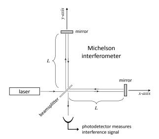
Michelson interferometer for detecting gravitational waves. The two mirrors and the beamsplitter are suspended so that they act as free masses.
